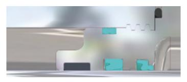
Zurcon\* U-Cup RU9 used as a single seal in a sealing system with a double-acting scraper.
