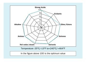
In tests, **Isolast**\* J9503 has shown considerably better compatibility over comparable competitor products, as seen in *figures 3 to 5*. All tests were carried out on standard 0-Rings size 214 (24.99 x 3.53 mm/.984 x .139 inches) and in accordance with test procedure DIN 53521.
