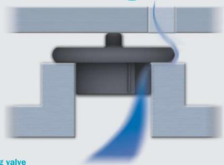
**NEW:** the reliable elastomeric venting valve
