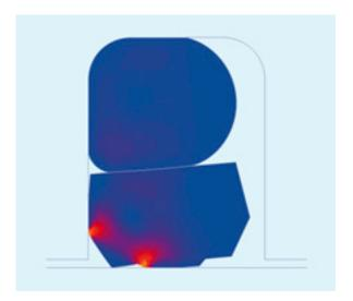
The fact that the profile is supported by a second edge restricts contact with the shaft, thereby significantly reducing friction and wear. The material used for the energising ring can be adapted to suit operating conditions. The angle on both sides of the polyurethane ring prevents extrusion into the extrusion gap.
