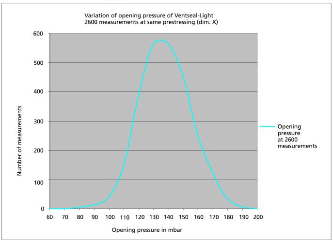
Figure 4 Distribution of the opening pressure values of the Ventseal-Light manufactured in the series tool
