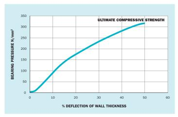
Typical deflection under load for a cylindrical bearing
