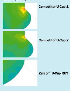
Zurcon\* U-Cup RU9 shows better extrusion resistance than standard U-Cups in the same hardware and service conditions.
