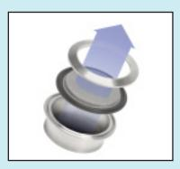
The  $V^2B$  vent gasket offers an additional answer for vacuum and pressure relief for pharmaceutical and food/beverage processing tank venting when airborne particulate removal is required. Using a 200 mesh screen combined with a 14 mesh screen of sintered construction, the  $V^2B$  vent gasket is a cost-effective alternative to expensive vacuum breakers and venting systems.
