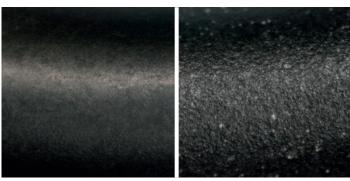
Surface of an uncoated seal (left) and of a seal coated with Flexcoat™ SF (right)
