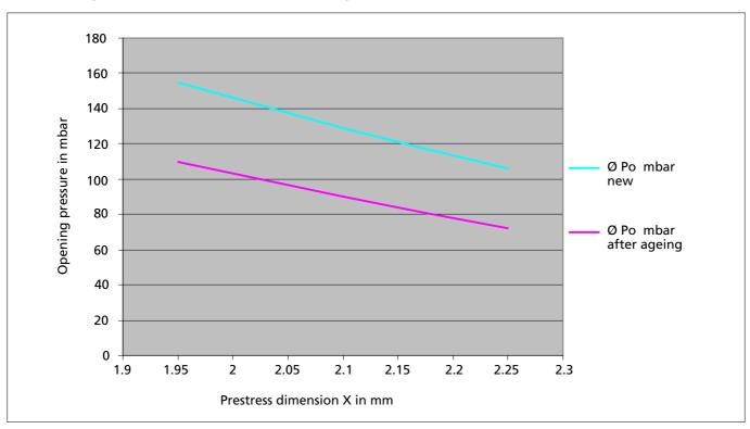
Figure 3 Opening pressure of Ventseal-Light manufactured in material E5501 depending on the prestress dimension X - new and after ageing
