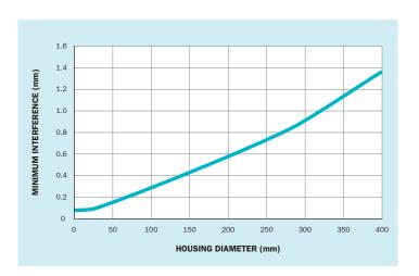
This interference is used with the housing and bush diameter machining tolerances to determine the bush outside diameter. The use of an interference fit to hold a bearing requires a reasonable machined tolerance on the housing bore, typically BS EN 20286-2:1993 H7.
