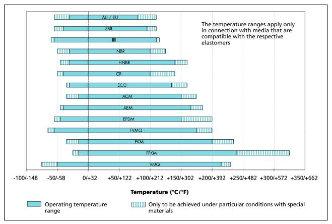
Figure 2 Temperature range of various elastomers
