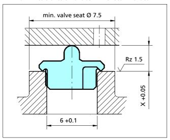
Figure 2 Ventseal-Light Installation
