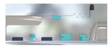
Zurcon\* U-Cup RU9 as a secondary seal in a "tandem design" sealing system with double-acting scrapers.
