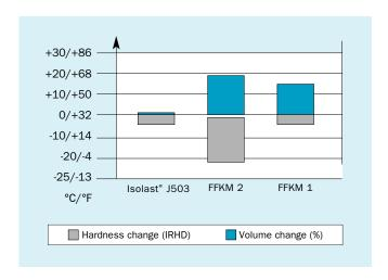
Figure 5: Immersion in pressurized steam at +200 °C/+392 °F
