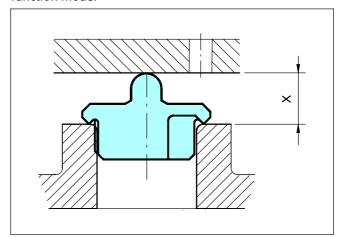
Figure 1 Ventseal-Light installed on a battery muff
