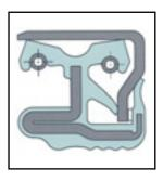
The **On-Road** version has one spring-energized sealing lip and three excluder lips, resulting in lower seal torque and higher allowable speed.
