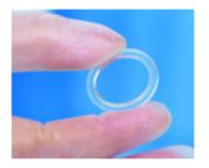
**Crystal clear elastomer**A specially developed translucent elastomer offers a sealing solution with an extremely low level of ionic impurities.
