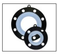
An Ansi Flex® (ANSI Flange 150#) gasket's contact surface is PTFE unitized to an EPDM rubber inner core. This totally bonded construction provides a PTFE gasket with the mechanical characteristics, including memory, of an elastomer gasket with exceptional steam resistance. An ANSI Flange 150# gasket is ideal for applications, such as PVC piping and glass lining pipings, where low seating stress is required.
